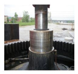
This picture was taken before we started the repair on one of two center pins. These pins were worn from many years of use. The repair consisted of building the material back up and then machining it back to size.
