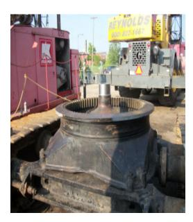
The finish product is in new condition and was repaired at about 10% of the replacement cost. The two center pins were finished in approximately one week, saving the customer costly down time.
